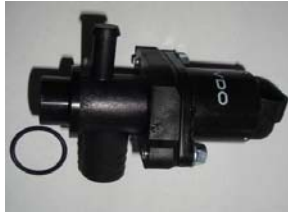
9356-0 Stepper with body, suit AU Tickford and dual fuel aftermarket kits.
