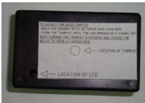
EFF001 Module start control & decel signal to AMS with LED Indicator
